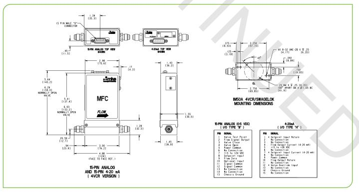
$\textit{Dimensional Drawing} - \textit{Analog 15 pin D for either 0 to 5 VDC or 4 to 20 mA I/O shown above with VCR fittings}^{\star}$
