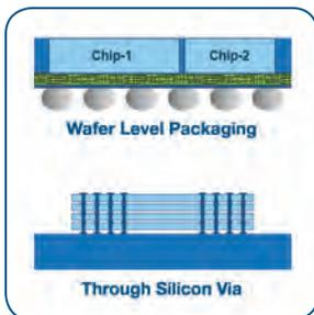
Through-Silicon Via (TSV) is the feature that enables 2.5D and 3D advanced packaging. Via pathways are short vertical columns through the silicon wafer or die that form electrical connection pathways. Vias enables smaller package sizes by removing the need for external wire bonds, support
