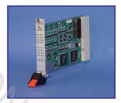
The SCOM-0800 and SCOM-0801 are designed as general-purpose serial communication cards with standard RS-232 and RS-485 ports. Protocol is jumper selectable per channel. The I/O and power signals are distributed through J2 rear connector. The board form factor, physical dimensions and BUS interface comply with CompactPCI® Specification PICMG® 2.0 R2.1.
