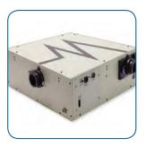
The spectrograph is a complete optical spectroscopy system offered by MKS. The optical design of the MKS family of spectrographs is based upon an asymmetrical in-plane Czerny-Turner monochromator. The spectrograph produces a flat image plane for use with multichannel detectors.
