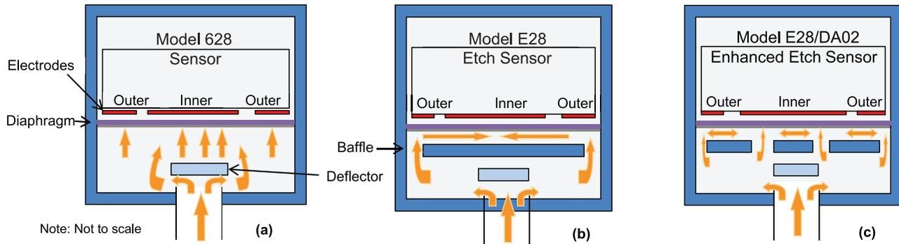
Figure 3 - Manometer baffle evolution
