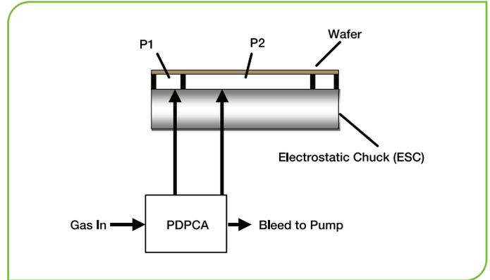
Figure 1 – Two Zone Backside Wafer Cooling
