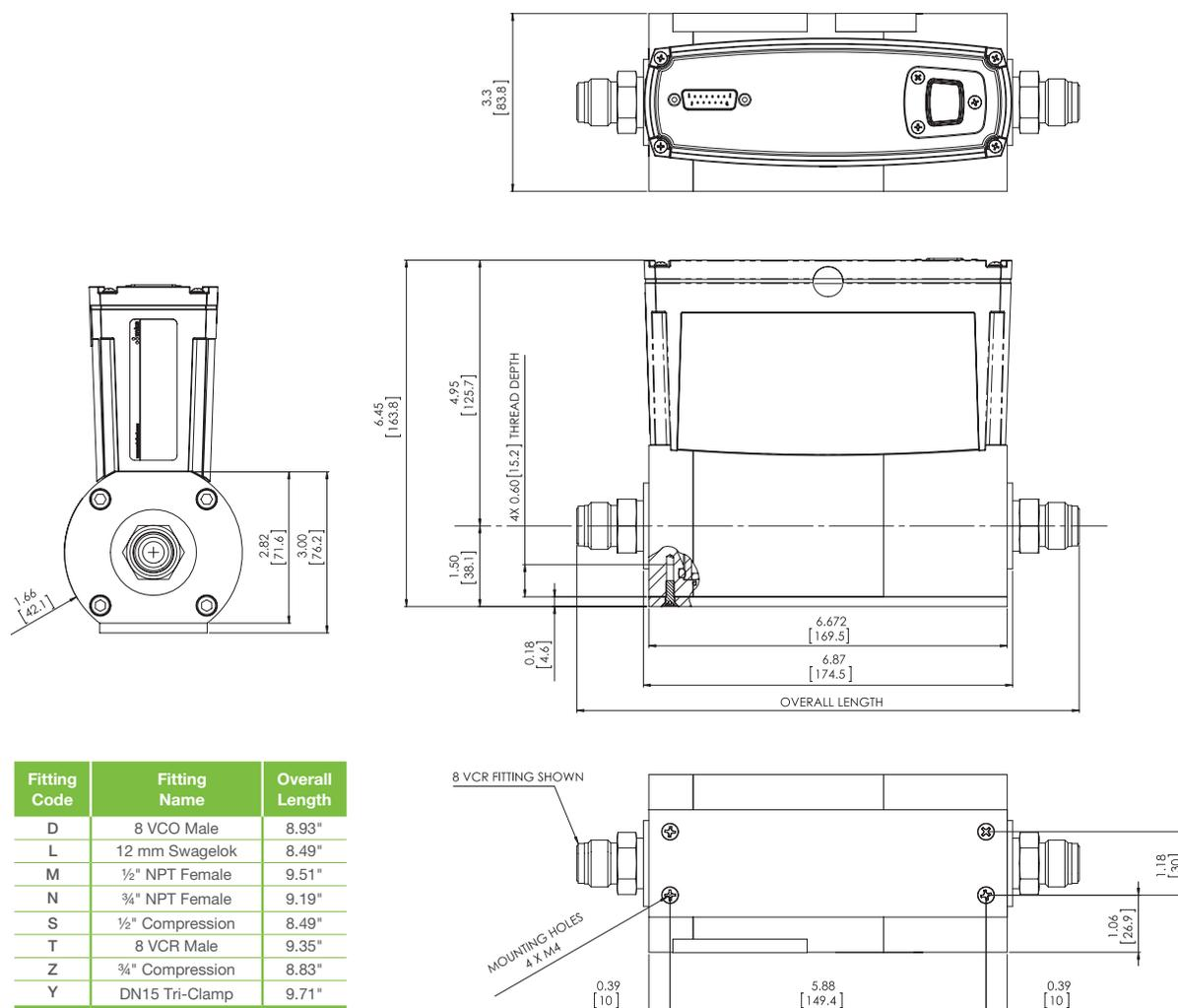
Unless otherwise specified, dimensions are nominal values in inches (mm referenced). \*See manual for additional I/O and fitting types. x.xx = ±0.020 tolerance
