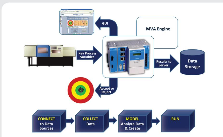
Figure 1. The SenseLink™ QM in-line quality detection system.
