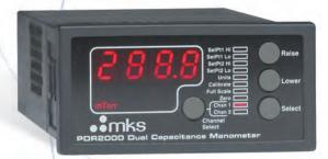
**Power Supply & Readout** — MKS offers a versatile, low cost solution for providing power and displaying pressure output values for the MKS Baratron® family of transducers. Up to two manometers may be operated from a single PDR2000. Readings are displayed on the front panel and are also available on demand via RS232 interface. Engineering units include Torr/mTorr or mBar/microBar.
