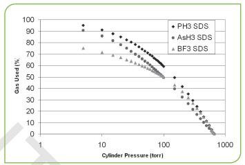
Figure 1 — SDS Gas Use Rate Efficiency
