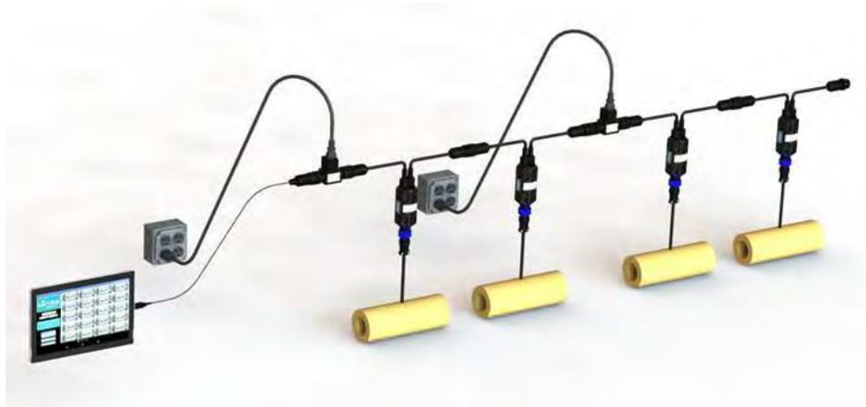
*Figure 9: Daisy Chain Heater Application, Dual/Multiple Power Drops*
