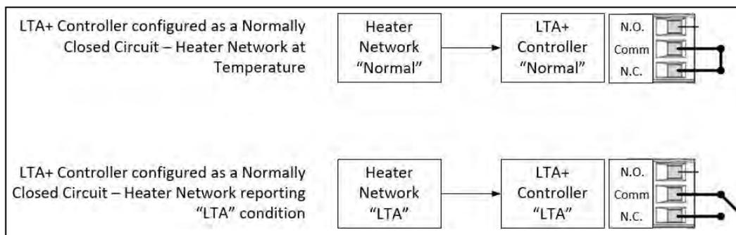
Figure 18: LTA+ Controller Process Control - Normally Closed Configuration
