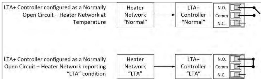
Figure 19: LTA+ Controller Process Control - Normally Open Configuration
