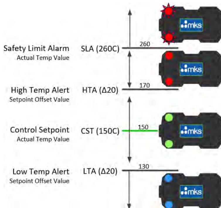
Figure 13: Series 49 LED 1 Display- most common conditions
