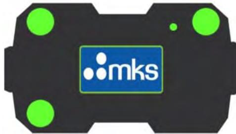
*Figure 15: S49UL LTA+ during the addressing cycle, showing a small green addressing LED*
