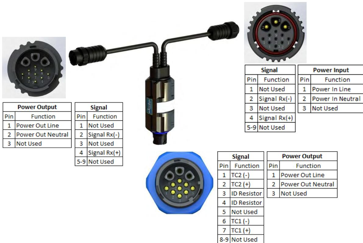
Figure 11: Heater Controller pin-outs
