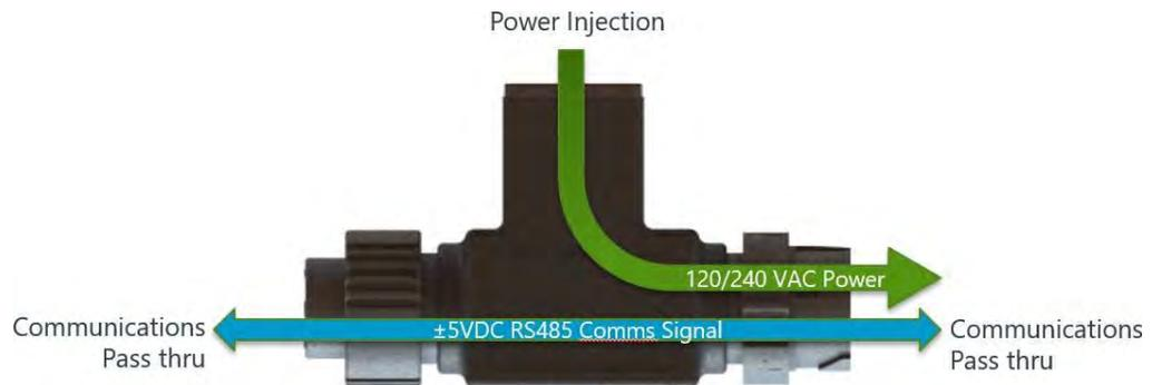
Figure 3: Power Adapter Power Injection and RS-485 Communications Pass Thru
