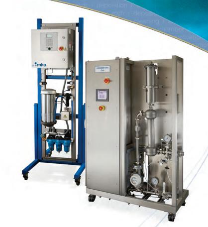
**Ozone Gas Destruct (OVS)** — Safety measures are of paramount importance to ensure the protection of personnel and equipment from unintended ozone exposure, especially the destruction of excess ozone gas. The OVS catalytic ozone gas destruct unit safely converts high levels of ozone into oxygen, reducing the ozone level down to detection limit and well below safety thresholds.
