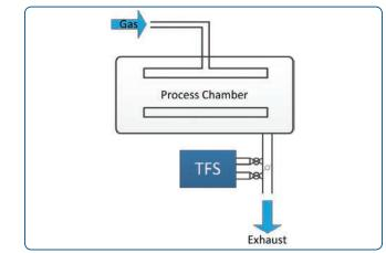
Figure 6 - Chamber clean endpoint detector
