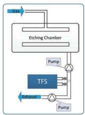
Figure 8 - One possible configuration for etching endpoint monitor with a TFS analyzer
