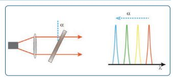
Figure 2 - Concept of using a tunable filter in spectroscopy. Rotation of the filter produces changes in the incident angle (left) which produces a varying wavelength transmission (right)
