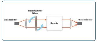
Figure 1 - Basic diagram of NDIR showing its major components
