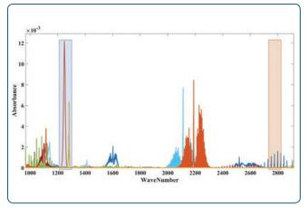
Figure 3 - Example of a dedicated TFS analyzer configuration. In this case, full range infrared spectra collected using an FTIR analyzer are shown. A TFS analyzer can be configured using 2 filters (highlighted ranges) to measure three independent gases.
