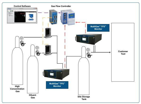
Figure 9 - Gas blending application of a TFS analyzer
