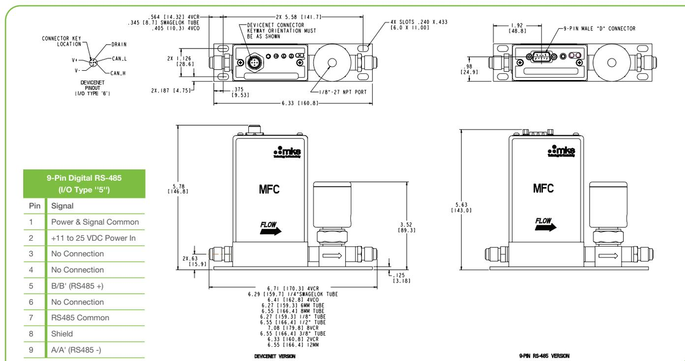
DeviceNet™ and RS485 with VCR fittings\* (\*see manual for additional I/O and fitting types). Unless otherwise specified, dimensions are nominal values in inches (mm referenced).
