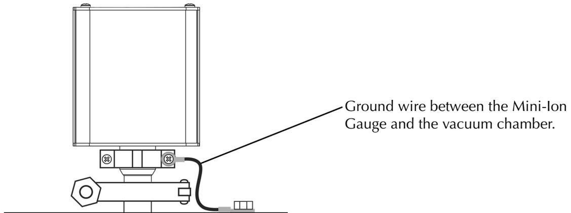
*Figure 4-2: Grounding the Mini-Ion Gauge to the Vacuum Chamber*
