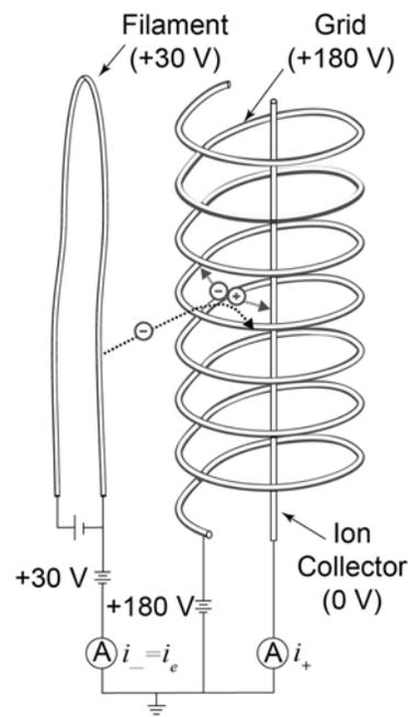
Figure 5-1: Typical Ion Gauge Schematic
