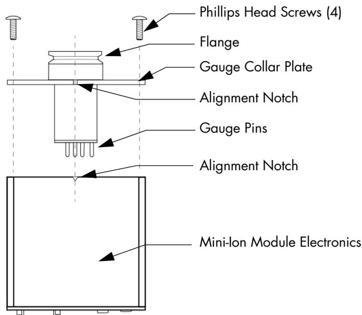
Figure 6-4 Mini-Ion Gauge Removal.
