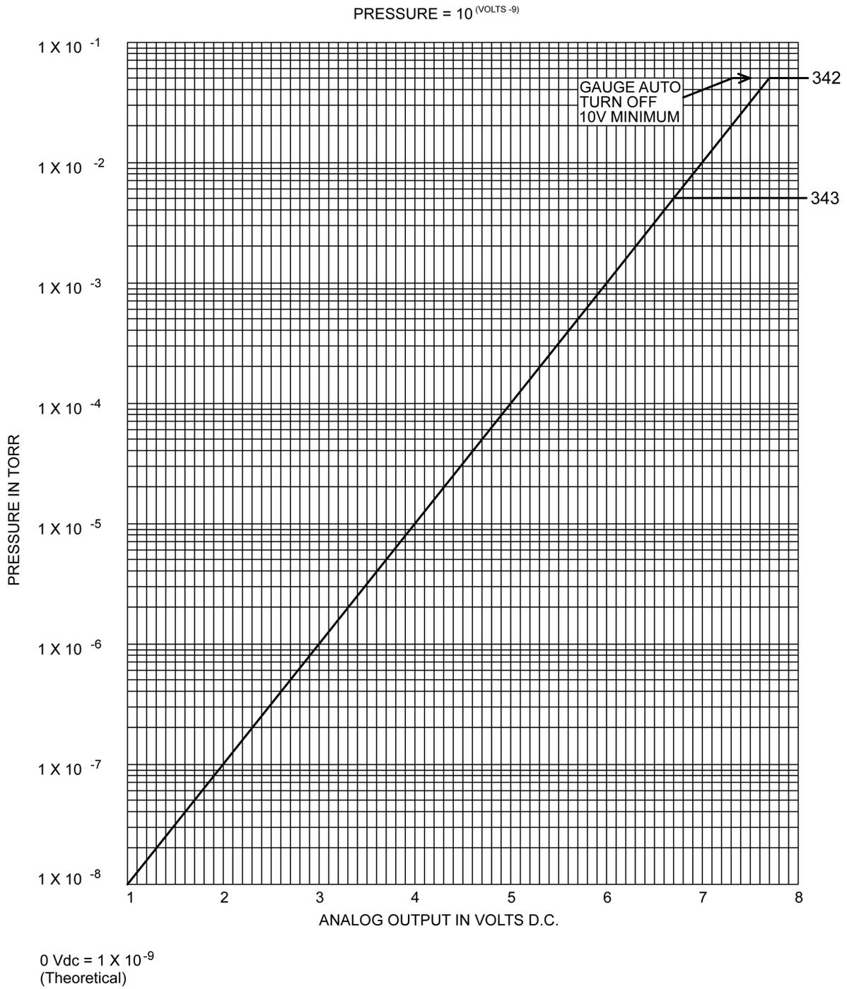
Figure 5-2: Analog Output in Volts dc
