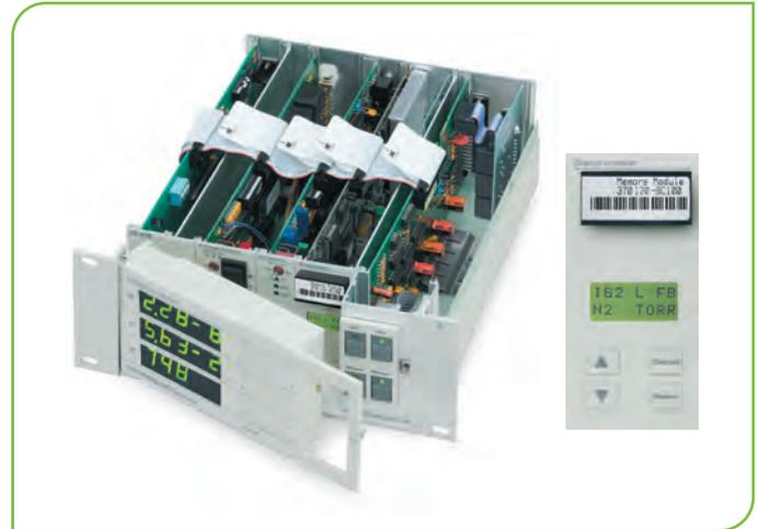
Vacuum Gauge Controller Cutaway
