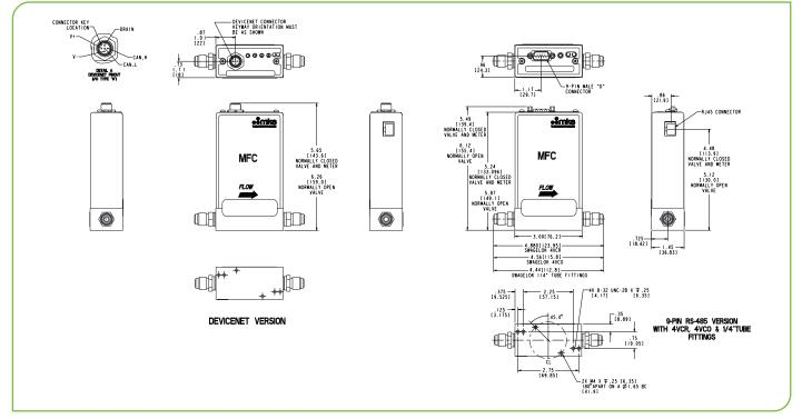
DeviceNet<sup>™</sup> and RS485 with VCR fittings<sup>\*</sup> (\*see manual for additional I/O and fitting types). Unless otherwise specified, dimensions are nominal values in inches (mm referenced).
