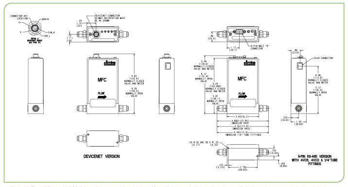
DeviceNet<sup>™</sup> and RS485 with VCR fittings\* (\*see manual for additional I/O and fitting types). Unless otherwise specified, dimensions are nominal values in inches (mm referenced).
