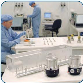
Bouncing electrons off a sample requires a tightly controlled vacuum environment to ensure image integrity resolution. To preserve electron beam integrity, the vacuum chamber must be completely free of scratches, aberrations, contaminants and properly vacuum sealed.
