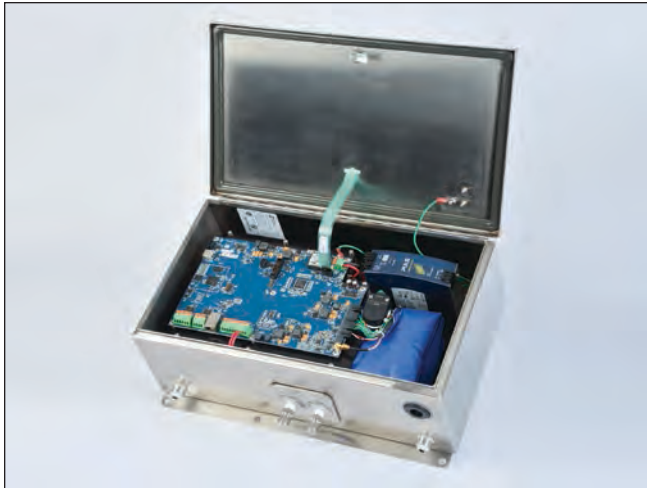
Tunable filter spectroscopy hydrocarbon gas analyzer.
