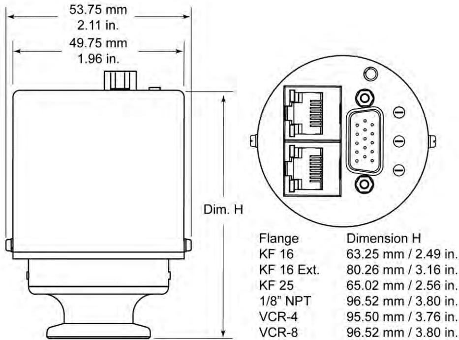
**972B Transducer EtherCAT Model Dimensions**
