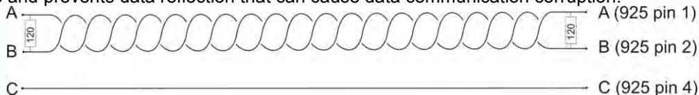
*RS-485 twisted pair cable run with 120Ω terminator resistors (925 with 15 pin connector)*
