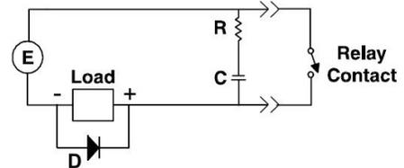
Note that  $R_{min} = 0.5 \Omega$  and  $C_{min} = 1 \times 10^{-9} F$ , D is a fast transient suppression diode.
