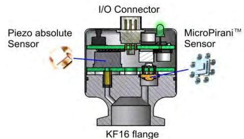
Both sensor elements are very robust and can withstand high G-forces and instant air inrush.
