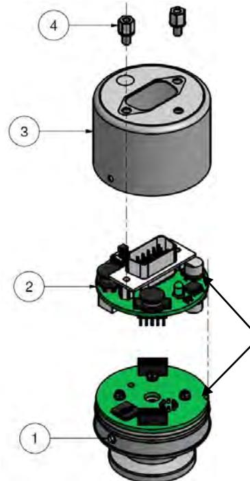
Printed circuit board alignment identification
