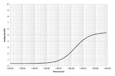
Analog out calibration = 8 (MKS Moducell 325)
