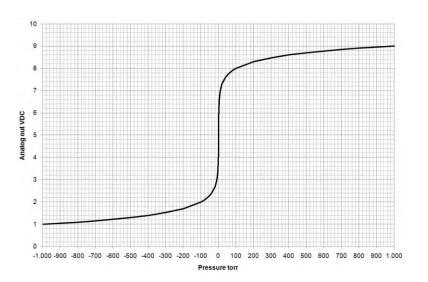
For positive pressure (V<sub>out</sub>>5 VDC)
