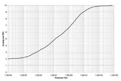
Analog Output calibration = 23 (MKS GP275 Emulation 9 VDC FS)
