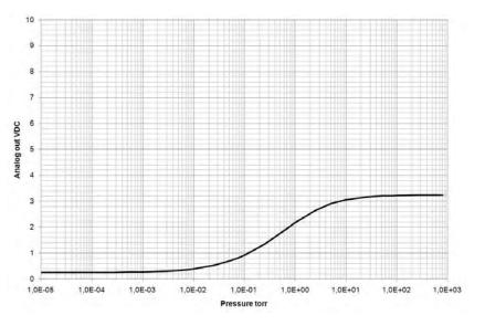
Analog out calibration = 9 (MKS Moducell 325, amplified 3 times)
