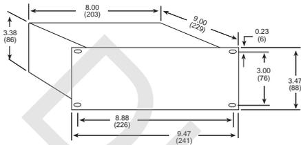
Note: Allow 2.5" (63 mm) clearance behind rear panel for connectors/cables.
