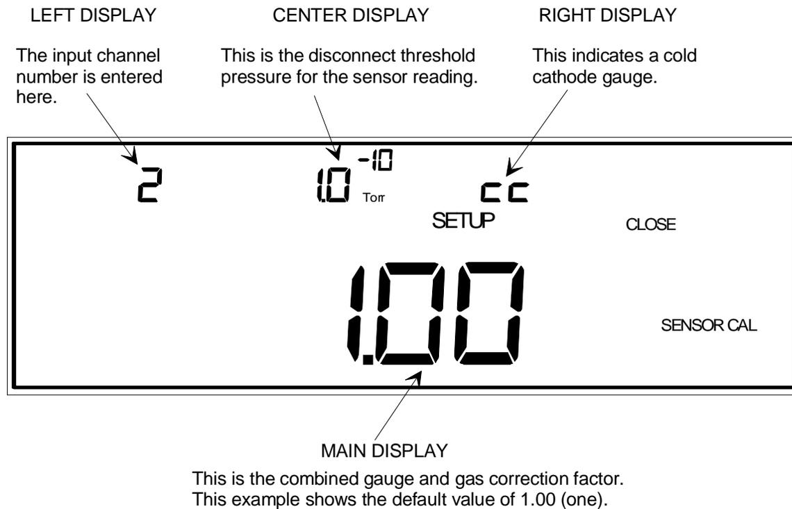
Figure 58: Sensor Calibration for Cold Cathode Gauges
