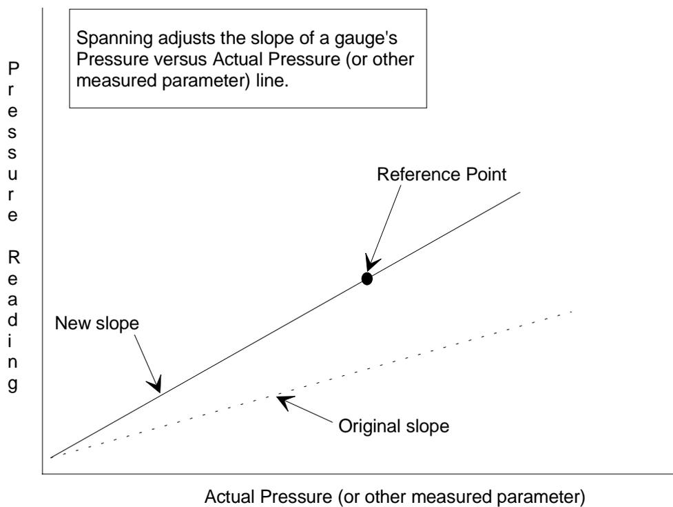
Figure 38: Spanning a Sensor with a Reference
