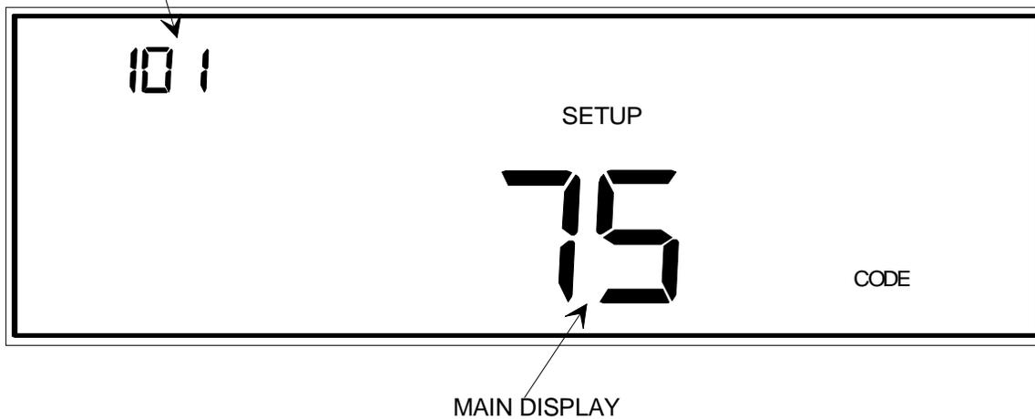
This is the display lag percent. The range for the lag percent is 1 to 100, where 100% is the highest display sensitivity. Use a high display sensitivity for very quiet applications only.
