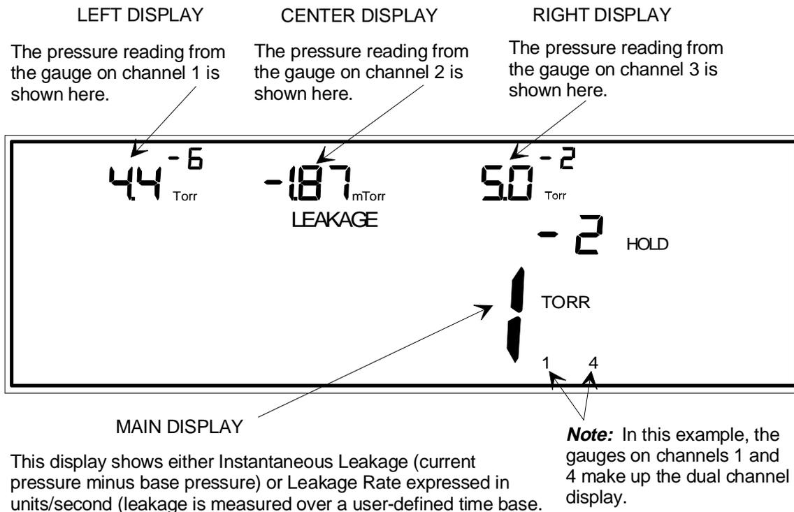
Base pressure is the pressure reading on a channel when Leakage Mode is first entered. Base pressure is obtained and stored for all active channels.
