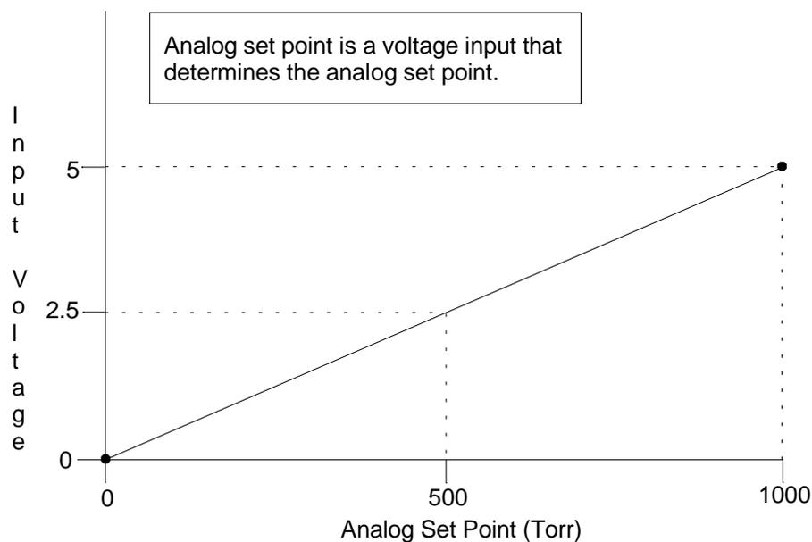
Figure 39: Graph Showing Analog Set Point Defaults
