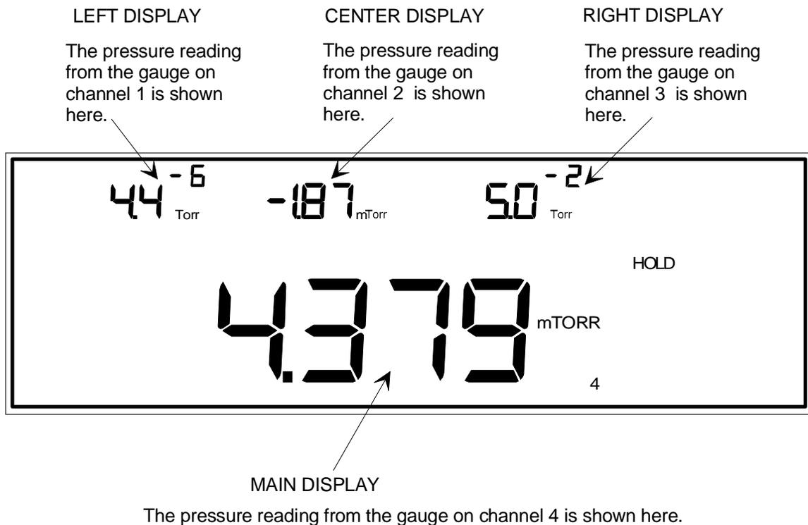
**Note:** It is possible to display the pressure reading from a gauge on any channel in the Main Display.
