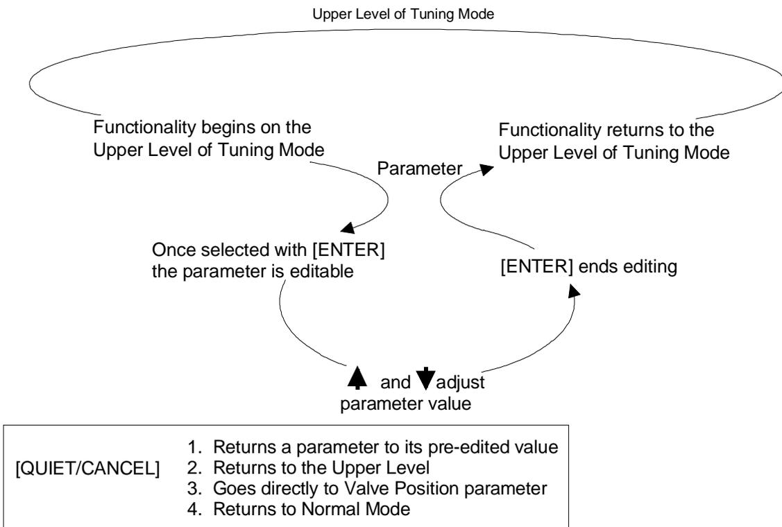
Figure 43: The Two Levels within Tuning Mode
