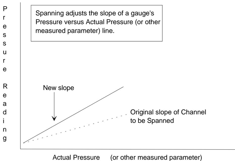
Figure 37: Spanning a Sensor
