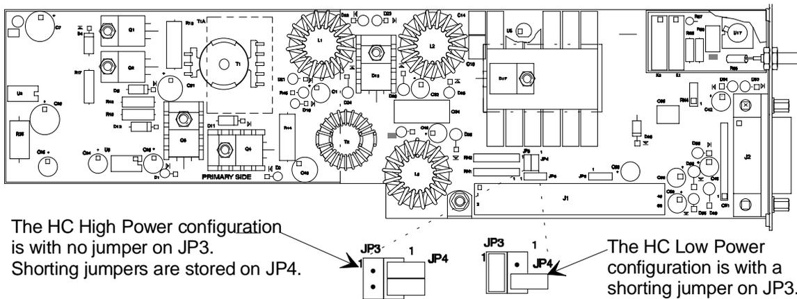
Figure 17: Jumper Placement on the Hot Cathode Board
