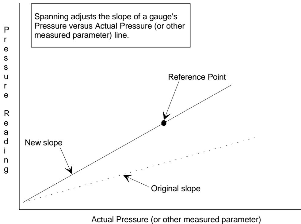
Figure 30: Spanning a Sensor with a Reference
