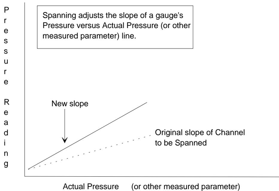
Figure 29: Spanning a Pirani-Type Sensor
