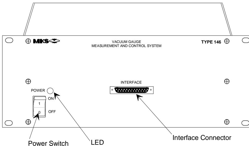
Figure 24: The Front of a Displayless 146 Unit
