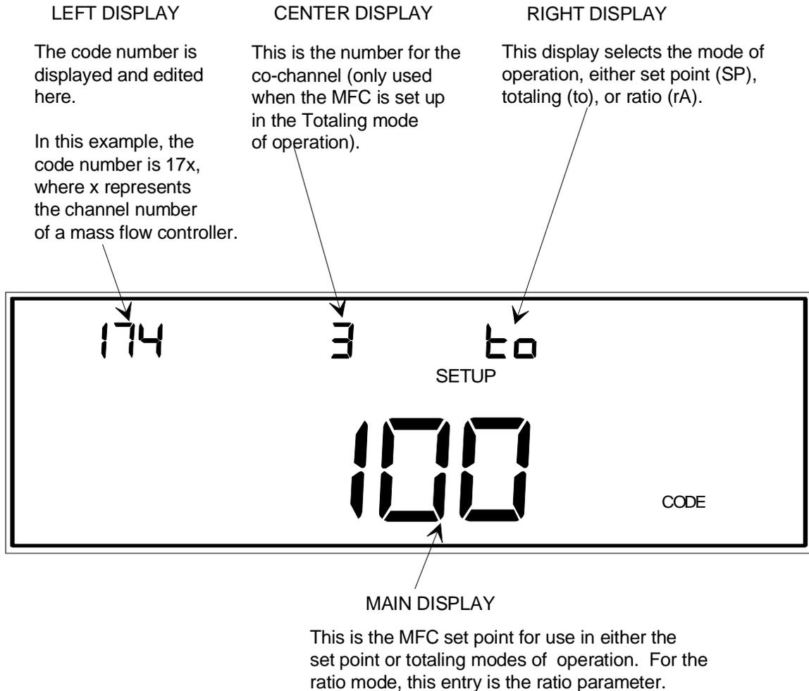
**Note:** The unit for the set point entry is sccm.
