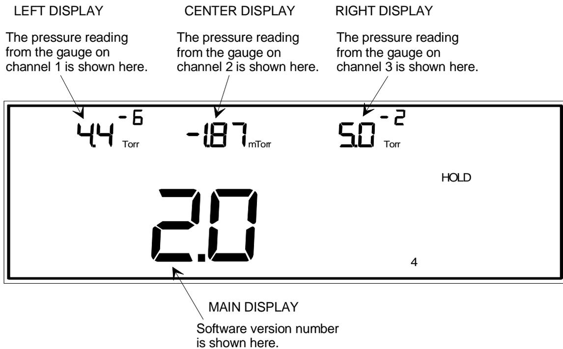
Figure 26: Software Version Number in Normal Mode
