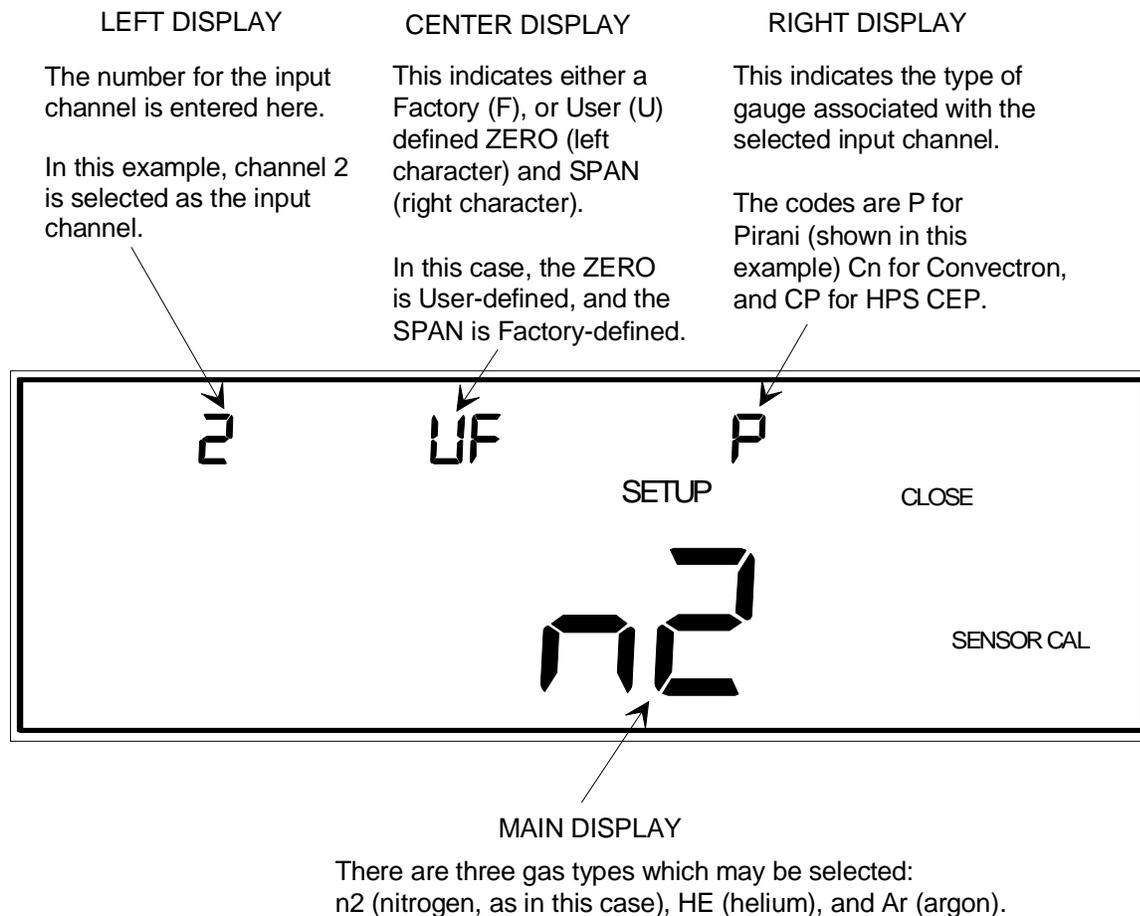
Figure 57: Calibration for Pirani and Convection Gauges
