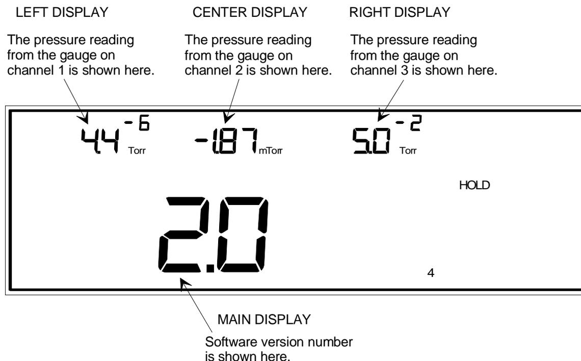
Figure 34: Software Version Number in Leakage Mode
