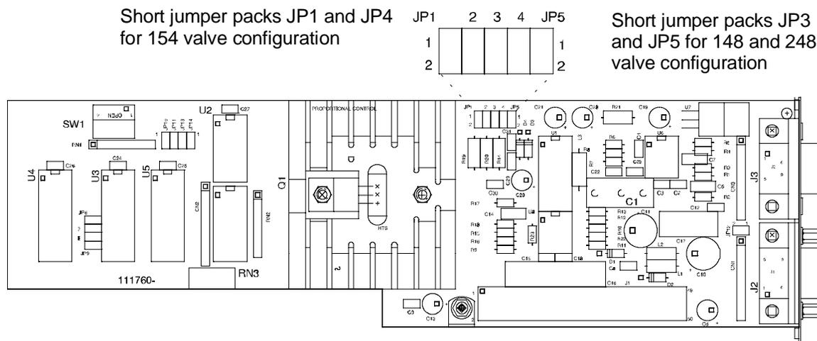
Figure 20: Jumper Placement on the Control Board
