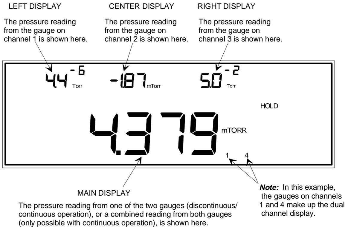
Figure 27: Dual Channel Display in Normal Mode
