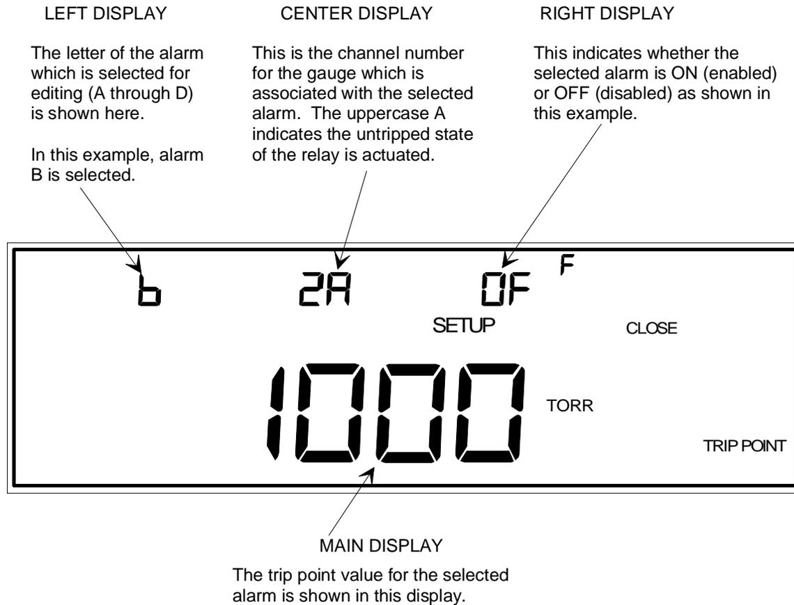
Figure 54: Display for Setting Alarm Trip Points
