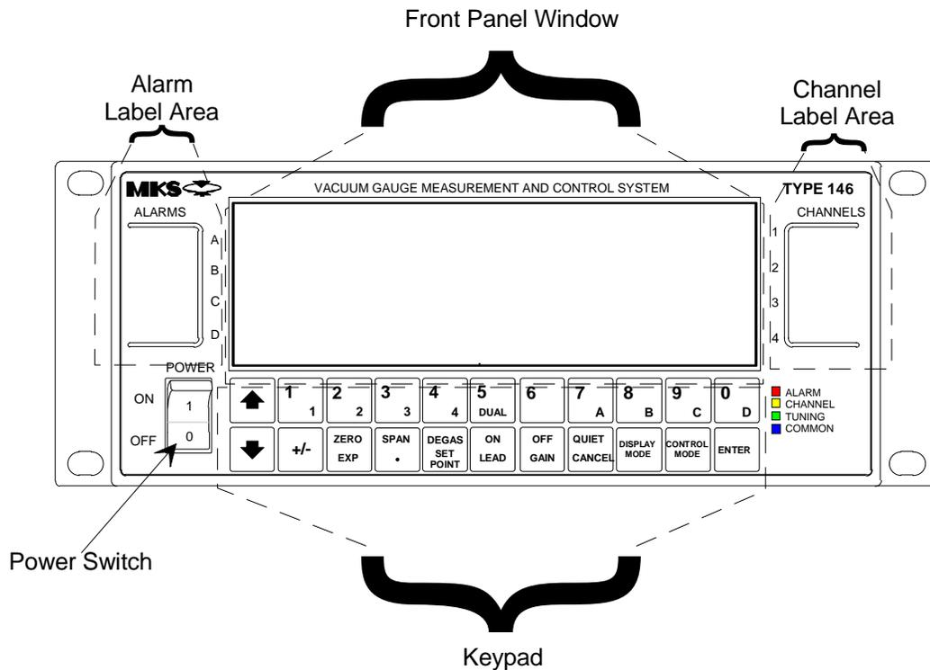
Figure 1: The Front Panel of the 146 Instrument
