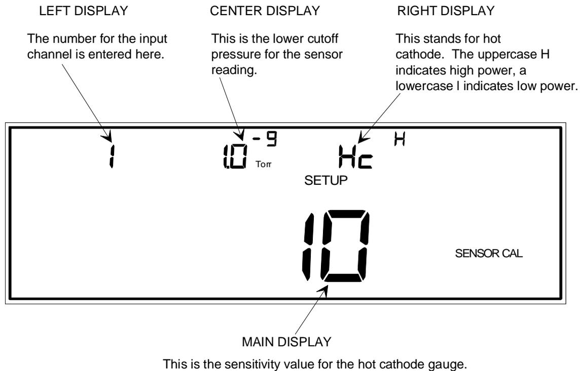
Figure 59: Sensor Calibration for Hot Cathode Gauges
