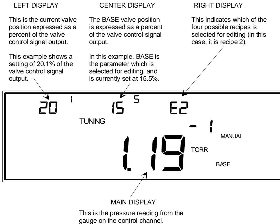
Figure 46: Adjusting the Base Valve Position
