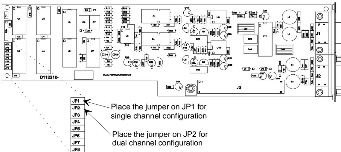
Figure 16: Jumper Placement on the Pirani/Convection Board
