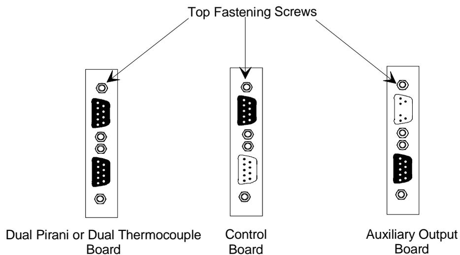
Figure 10: Fastening Screw Positions
