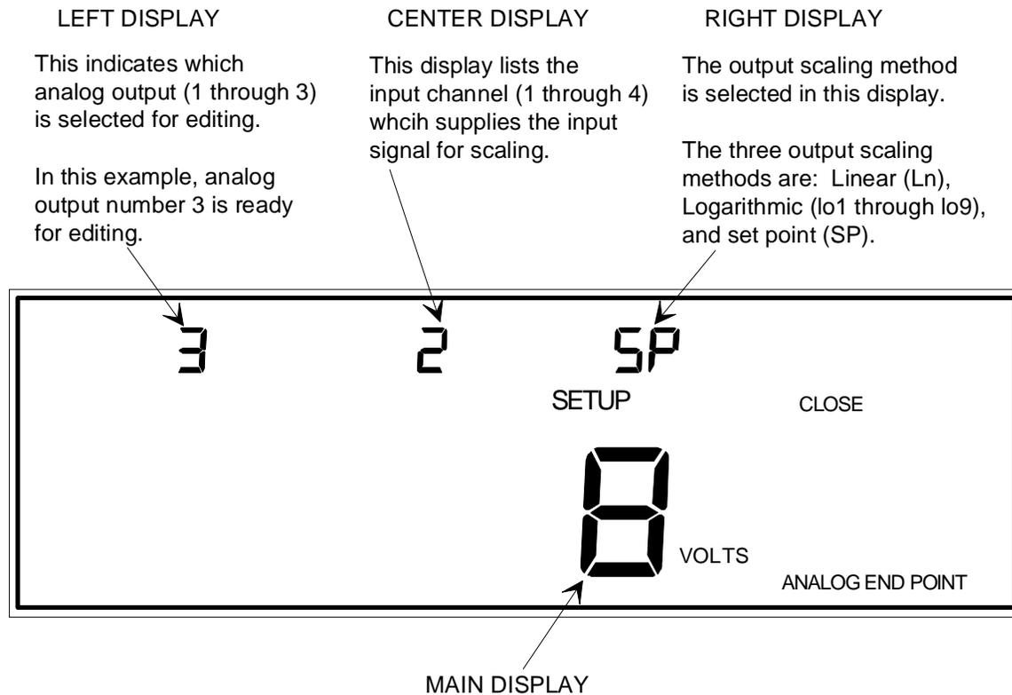
This display currently shows an output voltage of 8 Volts because the output scaling method selected in the right display is SP (set point). If either Ln or lo0 through lo9 (logarithmic) is selected as the output scaling method, the main display is used to enter the pressure value corresponding to the full scale output.
