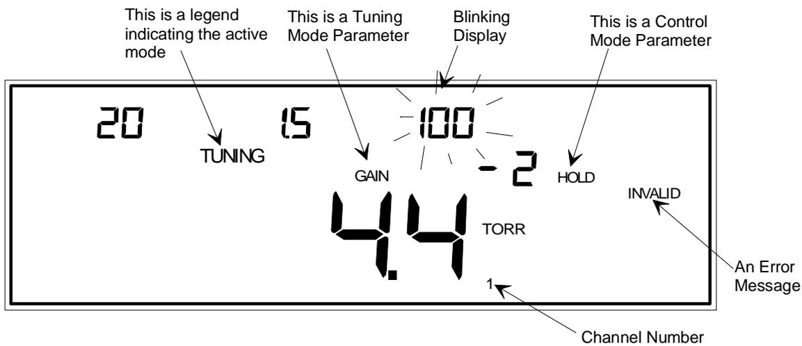
Figure 13: Explanation of the Front Panel Display
