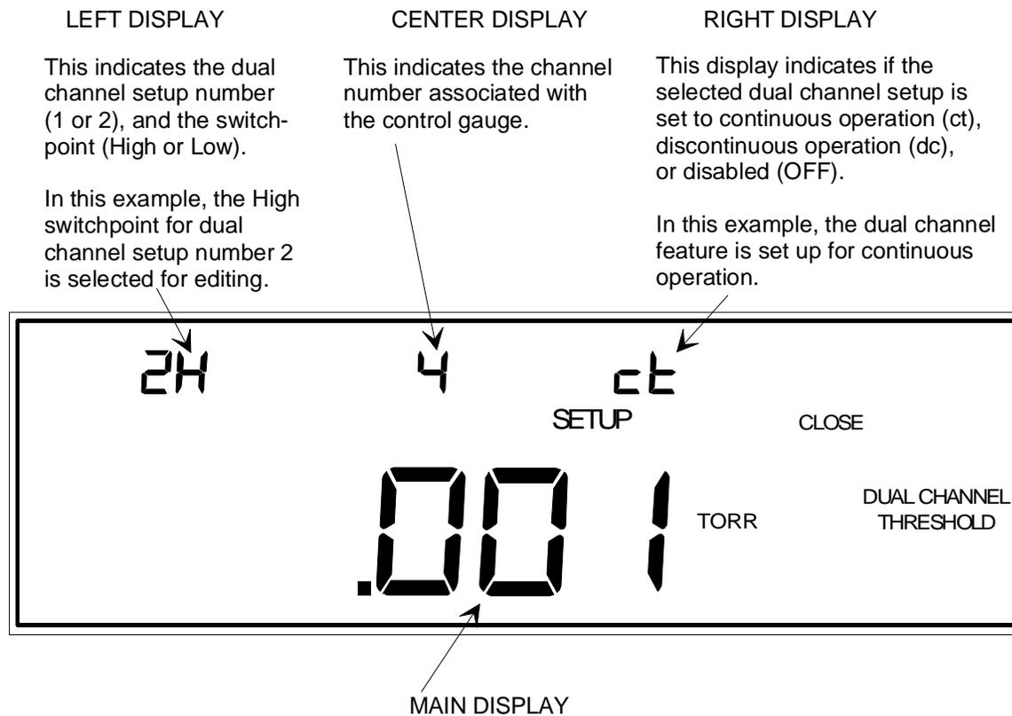
The switchpoint value for the selected dual channel setup is shown here. In this example, the value shown is the high switchpoint for dual channel 2.
