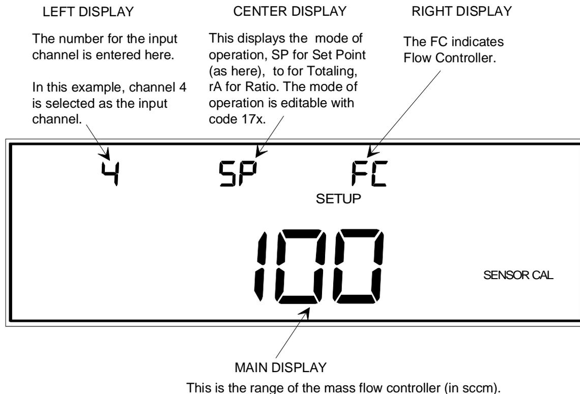
Figure 60: Sensor Calibration for Mass Flow Controllers
