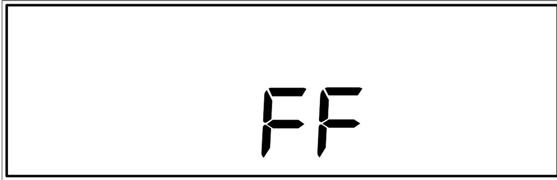
Figure 89: Rear Panel Output Test Display When all Bits are High
