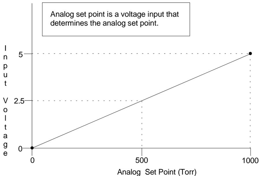
Figure 79: Graph Showing Analog Set Point Defaults
