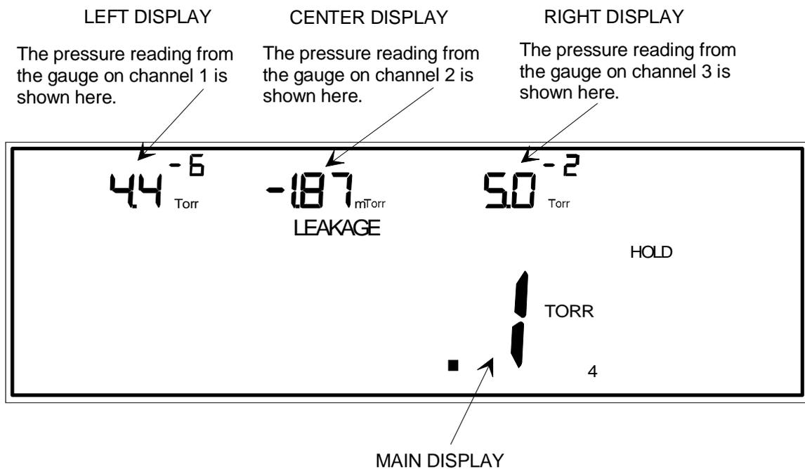
This is the leakage rate measured from the gauge on channel 4.
