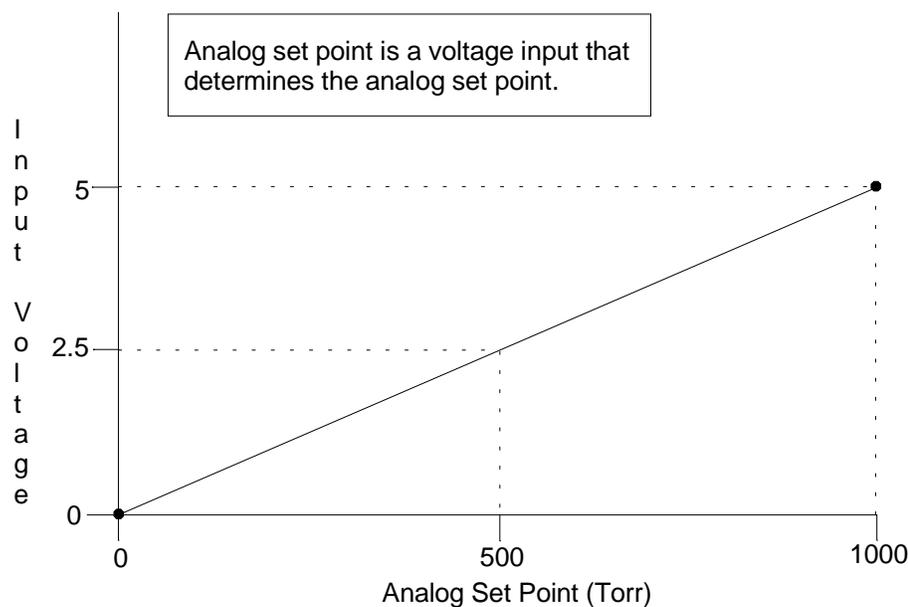
Figure 31: Graph Showing Analog Set Point Defaults
