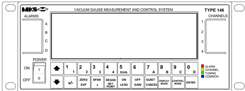
Figure 11: Front Panel of the Type 146 Instrument
