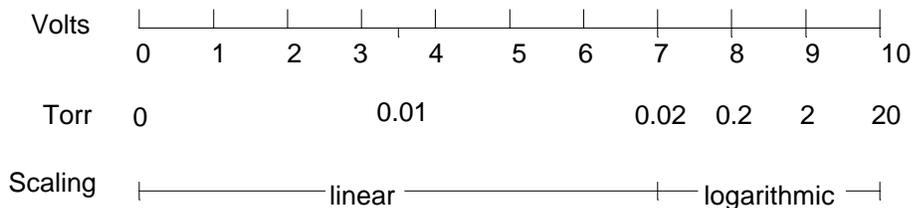
Figure 65: Linear and Logarithmic: Voltage versus Pressure
