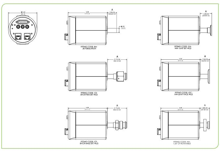
Unless otherwise specified, dimensions are nominal values in inches (mm referenced). For sensor code L, dimension A is 0.03" longer.
