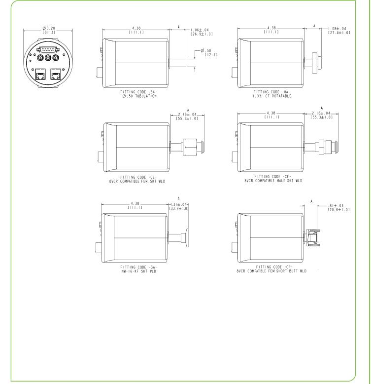
Unless otherwise specified, dimensions are nominal values in inches (mm referenced). For sensor code L or M, dimension A is 0.03" longer.
