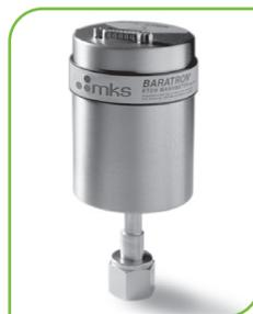
the sensor’s diaphragm measurement element. This greatly reduces the amount of zero drift in the Baratron capacitance manometer, which in turn improves the overall Cost of Ownership and process accuracy. These products are available in Full Scale measurement ranges as low as 0.02 Torr (0.27 mbar), and with either 15-pin D-subminiature (E27H and E28H) or 9-pin D-subminiature (E29H) electrical connectors.
