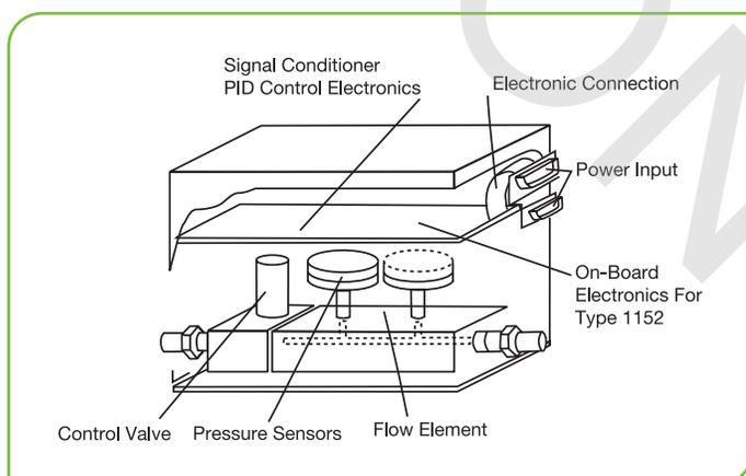
Figure 2 - Component Assembly
