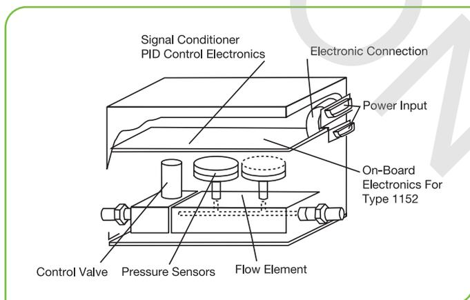
Figure 2 - Component Assembly
