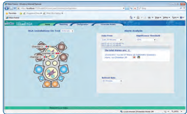
Figure 5 — TOOLweb RGA homepage screen for a tool with Vision 2000-P XD degas modules
