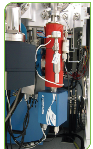
Microvision 2 installed as a 300mm Resist-Torr on a PVD tool degas chamber
