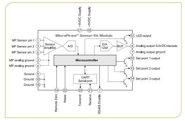
Electronics Module Pinout DIL 28 Pin Functional Block Diagram
