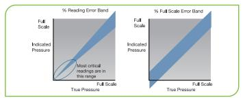
Figure 1 - Comparison of MKS repeatability expressed as percent of Reading transducer versus other percent of Full Scale transducers.
