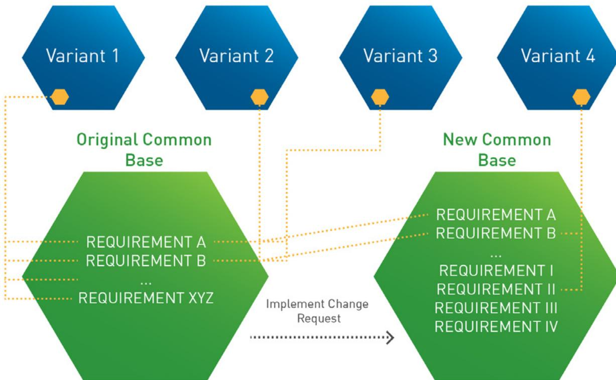
**Figure 2:** When a new version of the common base is produced, new variants may point to its requirements, but existing variants can keep pointing to the original version of the common base to preserve their certification until it is determined that a given variant is ready to inherit the change. As an architectural point, requirements that don't change in the new common base are just pointers to the same requirements in the original common base.
